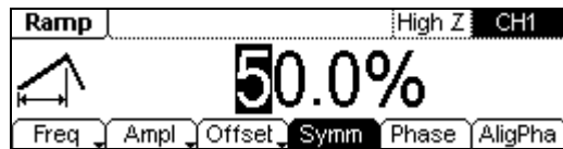
Figure 2-10 Ramp Signal Parameter Setting Interface
